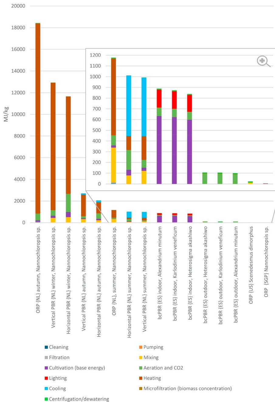
**Fig. 4.** Electricity use of the subprocesses in the cultivation of microalgae biomass in MJ/kg of dry microalgae biomass.
